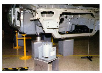
The MODAL 50A (and multiples thereof) is ideal for exciting structures smaller than say, a full-size automobile. Total vehicle modal tests on anything larger (truck, jet, even a space shuttle) requires multiple MODAL 50A's or the MODAL 250A.
